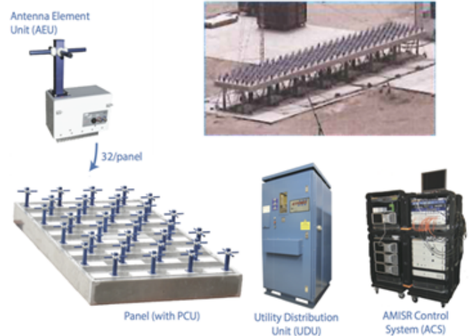
Fig. 1. AMISR-14 components.
